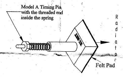
To use, assemble tool as illustrated and press into timing gear hole until felt edge can be placed easily against the radiator. Using a crank of fan/pulley method, turn the rotor until the pin seats itself in the timing gear indentation. The EZ SET tool serves as the third hand you need for this procedure.
